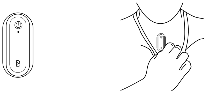
Image 6: Placement and positioning of the Bodystar BD1 on thorax
